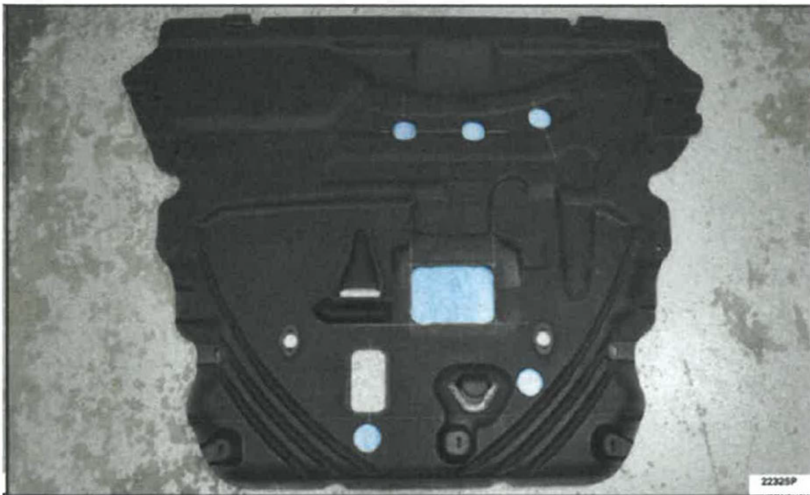
Figure 1: Image from the Defendants', FORD US and/or FORD Canada, letter to its dealers demonstrating the under-engine shield modification, with additional drainage holes highlighted in blue, as part of the required “fix” on all Affected Class Vehicles.
